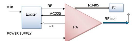
GME1R12 consists of two standard 19 "chassis, arranged vertically. The top is the exciter part (single and double exciters are optional), and the bottom is the 5U power amplifier unit. There is a lightning protection device and input switch at the back of the cabinet.
