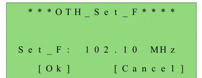
In this menu interface, the operating frequency of the transmitter is set at the numerical position. When the cursor is moved to "OK" and the confirm button is pressed, the operating frequency of the transmitter is set, which is used for calibrat of the detection system. And it will be displayed in the "SYS" menu.
